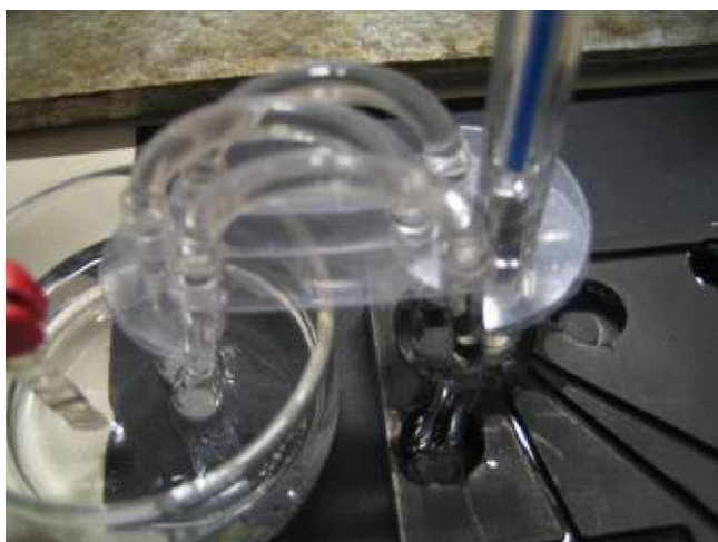
Fig. 7. From the reference/working electrode (right) compartment separated counter electrode (right); Separation was realized by the use of three electrolyte bridges (middle).
