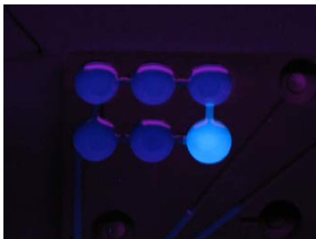
Fig. 10. Dye collection/concentration capability of the vial channel relief. After 40 min the dye starts diffusion in the neighbouring vials. Reflections of the ultra violet lamp on the liquid surface in each vial were removed in the high-throughput setup by the use of a band elimination filter
